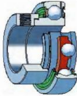
Y-bearing with eccentric locking ring, inner ring extended at one side
